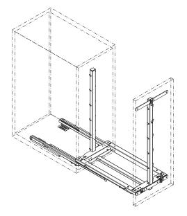
**LB** = Clear inside carcase width: ≥ carcase width **B**-40 mm
