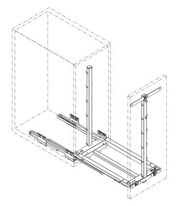
**LB** = Clear inside carcase width: ≥ carcase width **B**-32/38 mm
