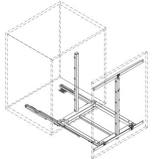
**LB** = Clear inside carcase width: ≥ carcase width **B**-40 mm
